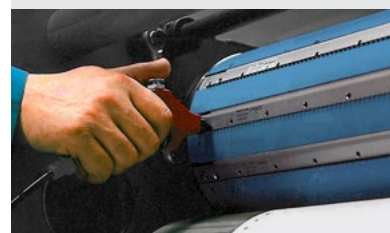
Cross perforation cylinder with pneumatical quick change bars.
