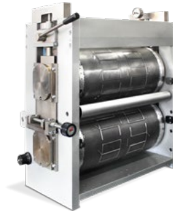
Creasing module with quick lift-device and wedge adjustment for the regulation of the crease depth, equipped with solid, segmented or magnetic creasing cylinders.
